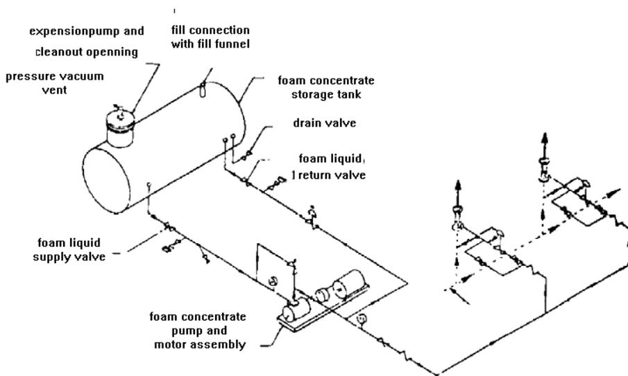
**BALANCED PRESSURE PROPORTIONING WITH MULTIPLE INJECTION POINTS (METERED PROPORTIONING) Fig. 9B (VERTICAL)**
