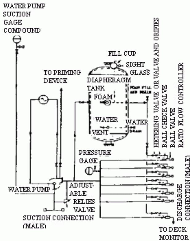
**PRESSURE PROPORTIONING DIAPHRAGM TANK METHOD**
