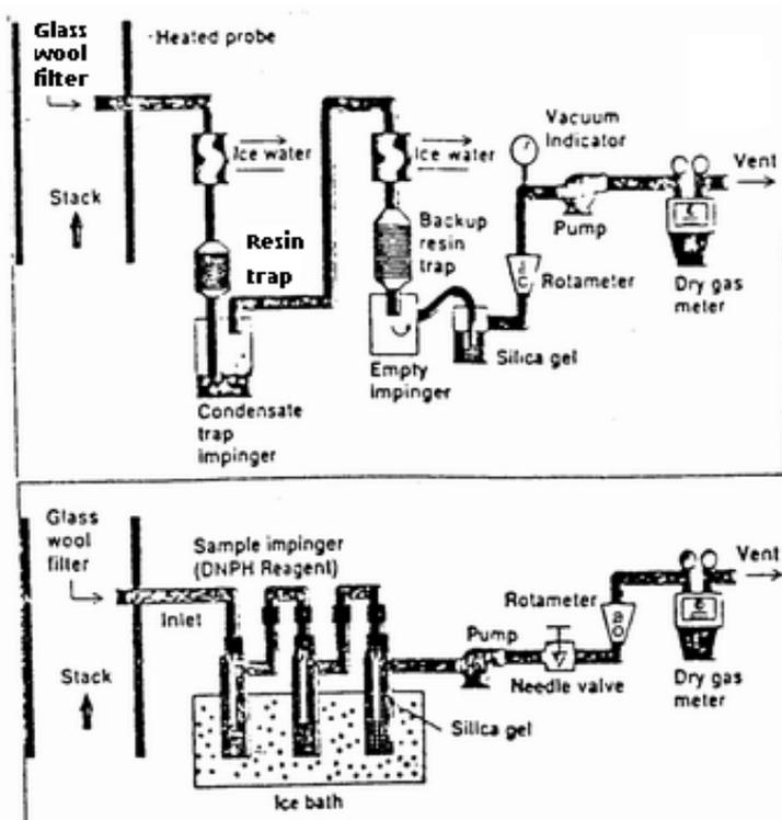
**SAMPLING TRAINS FOR VOLATILE ORGANICS (PHOTO AND TOP SCHEMATIC) AND A "WET IMPINGEMENT" METHOD FOR FORMALDEHYDE**
