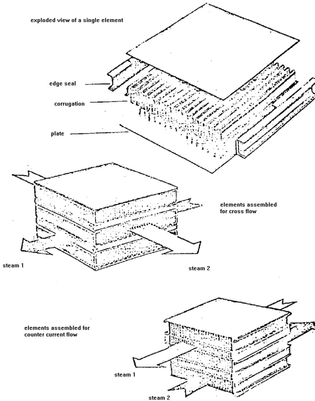
**PLATE FIN EXCHANGER ASSEMBLY**
