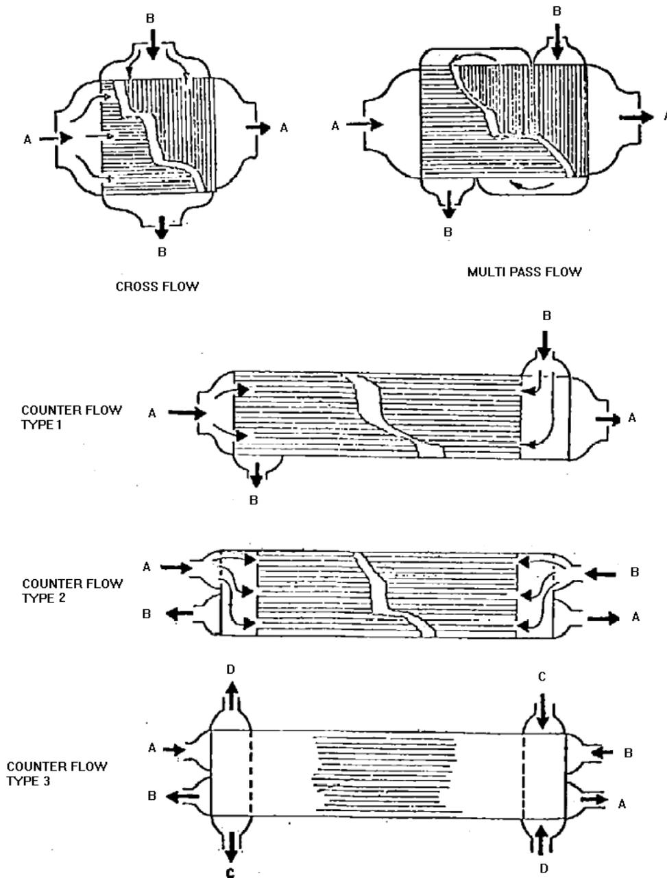
PLATE FIN EXCHANGER FLOW ARRANGEMENTS
