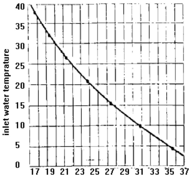
**AIR RELEASED FROM WATER kg air /1000 m<sup>3</sup>/h WATER**
