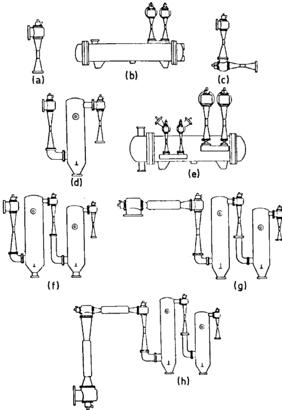
COMMON TYPE OF EJECTOR UNITS
