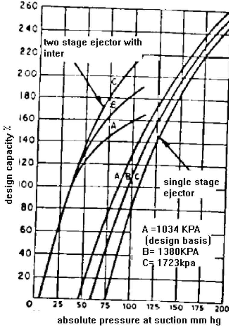
EFFECTS OF EXCESS STEAM PRESSURE ON EJECTOR CAPACITY
