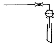
Telescopic loading lance with ball swivel and hand operated loading valve.
