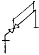
Articulated loading arm with hold-open hand-operated loading arm valve for white and black oil products.
