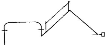
Boom type articulated loading arm with self-sealing coupling.
