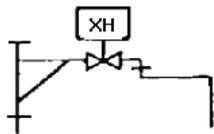
Short range boom type loading arm with hold-open hand-operated loading arm valve controlled by a hand-operated hydraulic system for black oil products.
