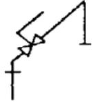
Articulated loading arm with stay-open hand-operated loading arm valve for white and black oil products.
