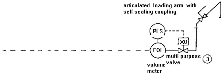
LOADING OF BULK ROAD VEHICLES BY METER-AUTOMATICALLY CONTROLLED
