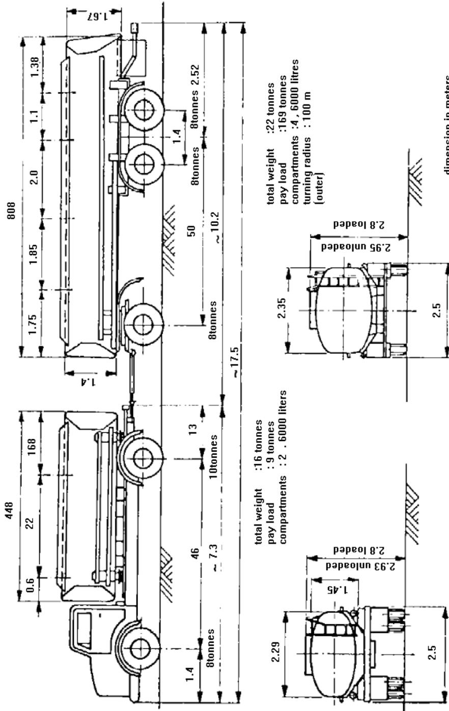
TYPICAL BULK ROAD VEHICLE WITH TRAILER
