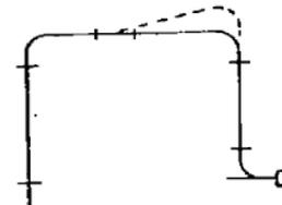
Hinged joint type hose loader with self-sealing coupling.
