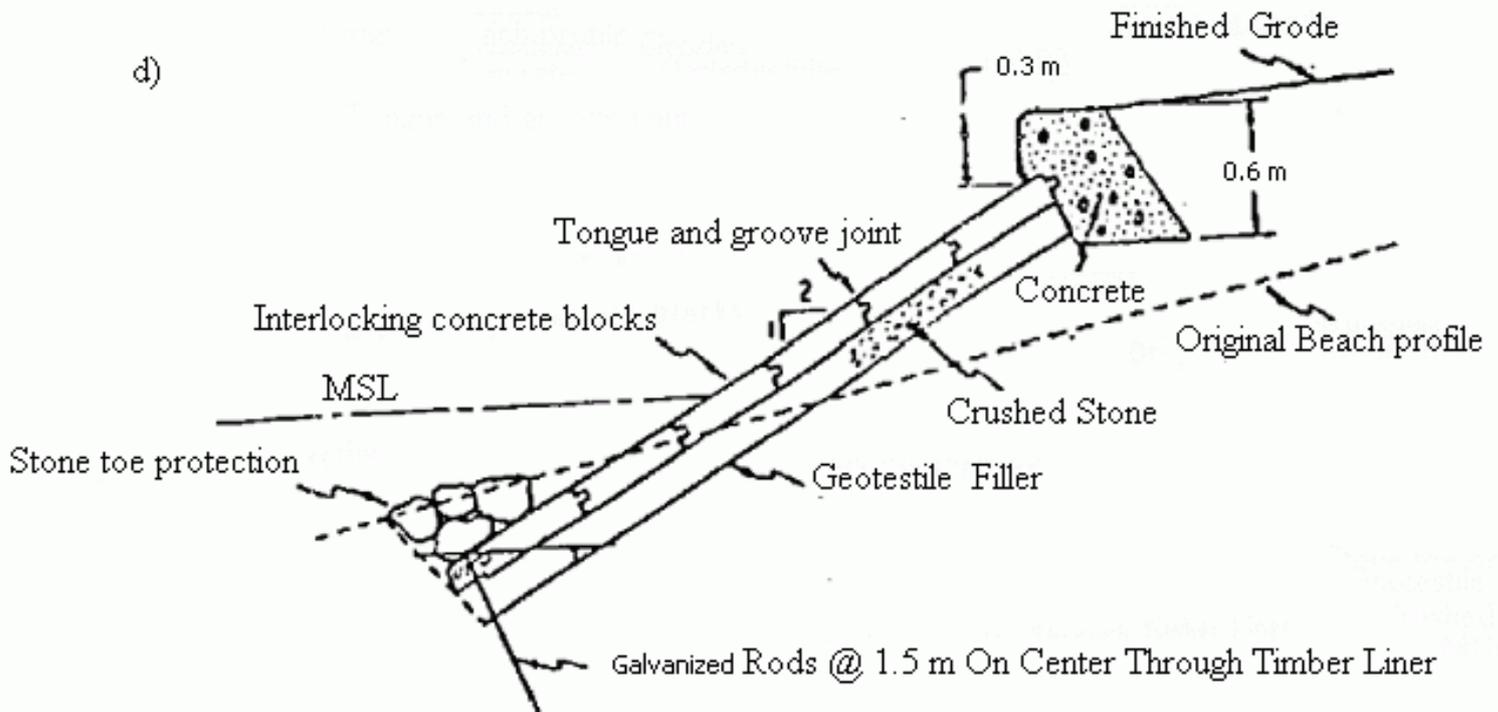
c) & d): Interlocking Concrete-Block Revetment
