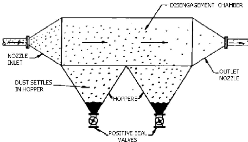
**EQUIPMENT FOR PARTICULATE REMOVAL (GRAVITY SETTLING CHAMBER)**
