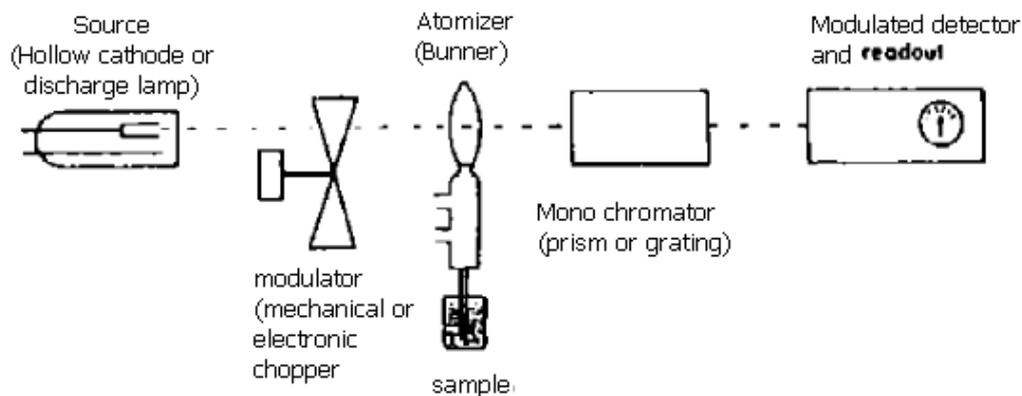
**SCHEMATIC DIAGRAM OF ATOMIC ABSORPTION SPECTROMETER**
