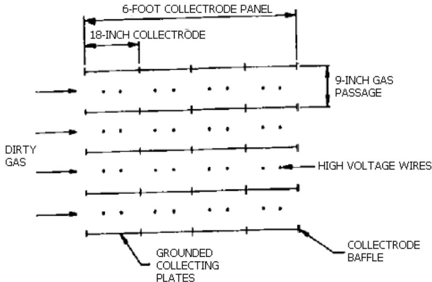
**CROSS SECTION OF FOUR-GAS-PASSAGE COLLECTRODE MODULE**
