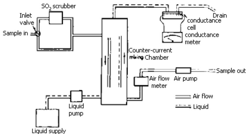
**COUNTER-CURRENT TYPE SULFUR DIOXIDE CONDUCTIMETRIC ANALYZER**
