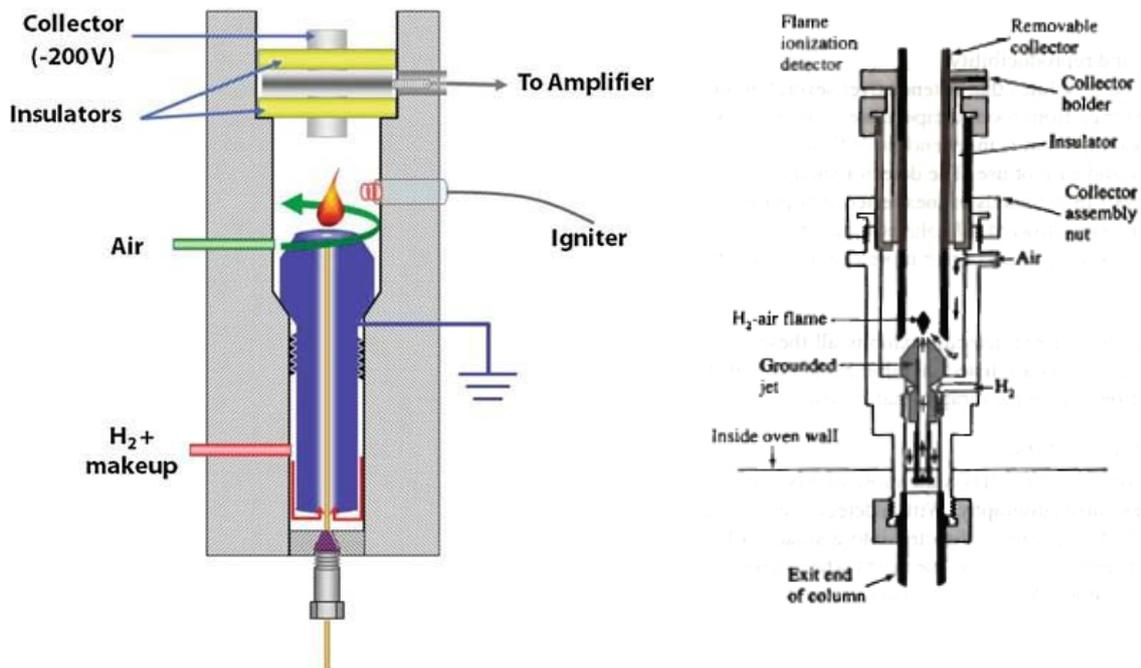
**FLAME IONIZATION DETECTOR (FID) FOR THE DETECTION OF HYDROCARBON**
