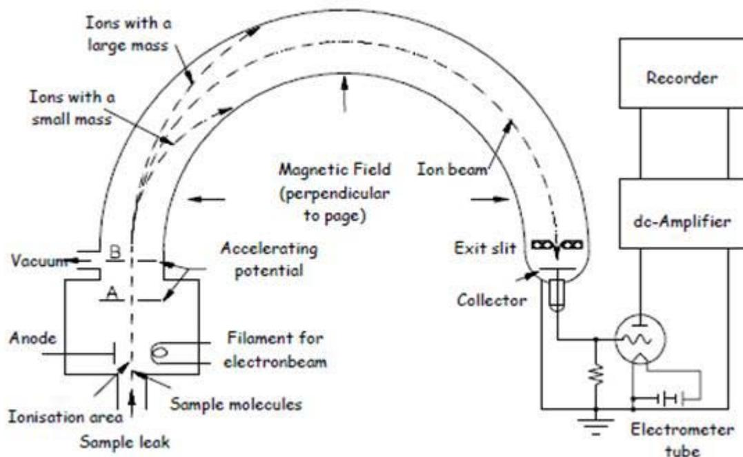
**SCHEMATIC DIAGRAM OF AN ANALYTICAL MASS SPECTROMETER**
