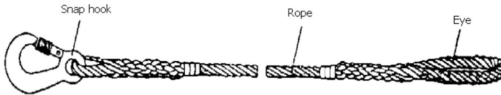
**EXAMPLE OF LANYARD (ILLUSTRATING A ROPE LANYARD WITH SNAP HOOK AND EYE)**
