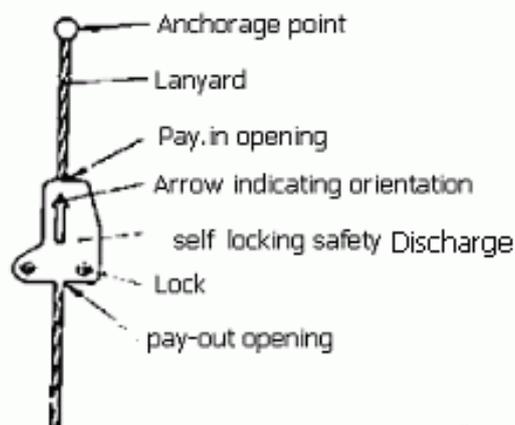
**EXAMPLE OF A SELF-LOCKING SAFETY ANCHORAGE ON A LANYARD**
