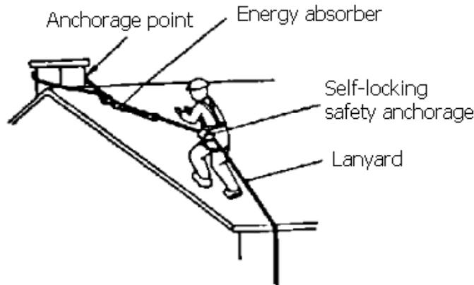
**EXAMPLE OF A SELF-LOCKING SAFETY ANCHORAGE ATTACHED DIRECTLY TO THE BELT**
