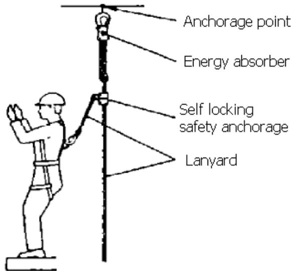
**EXAMPLE OF A SELF-LOCKING SAFETY ANCHORAGE WITH A LANYARD**
