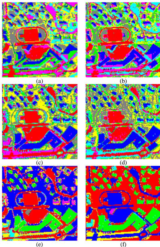
Fig. 5. (a) Result of applying FCM using Euclidean distance on hyperspectral data. (b) Result of applying FCM using Euclidean distance on derivative of hyperspectral data. (c) Result of applying FCM using cosine distance on hyperspectral data. (d) Result of applying FCM using cosine distance on derivative of hyperspectral data. (e) Result of applying fuzzy relational clustering on hyperspectral data. (f) Result of applying fuzzy relational clustering on derivative of hyperspectral data.
