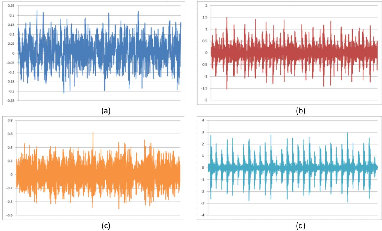
Figure 2. **Vibration signals acquired from four states of bearing. (a) Normal bearings (NB), (b) Outer race fault (ORF), (c) Inner race fault (IRF), (d) Ball fault (BF).**
