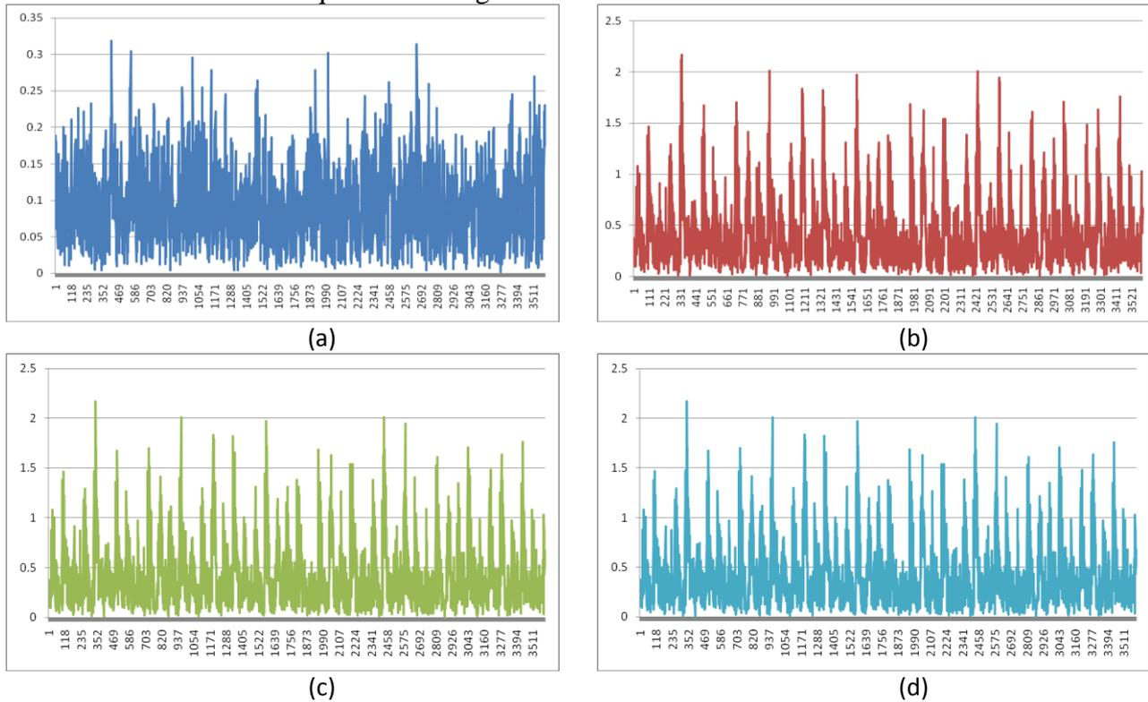
Figure 2. Envelope analysis of raw signal in four conditions. (a) Normal bearings (NB), (b) Outer race fault (ORF), (c) Inner race fault (IRF), (d) Ball fault (BF).
