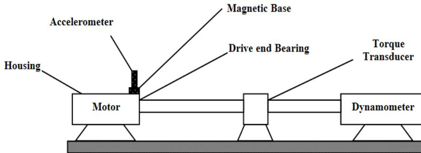
Figure 1. Schematic of Experiment System.
