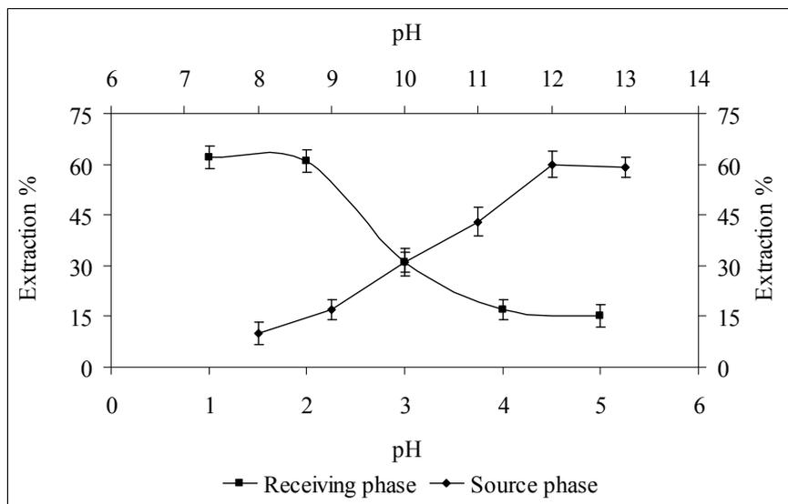
**Figure 1.** The effect of pH of source and receiving phase on the extraction efficiency. Extraction conditions:  $C_{TAM}$ ,  $50 \text{ ng}\cdot\text{mL}^{-1}$ ; SP, 15 mL; RP, 25  $\mu\text{L}$ ; stirring rate, 1000 rpm; extraction time, 60 min.
