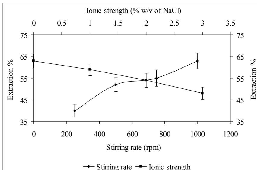
**Figure 2.** The effects of salt addition and stirring rate on the extraction efficiency. Extraction conditions:  $C_{TAM}$ ,  $50 \text{ ng}\cdot\text{mL}^{-1}$ ; SP,  $15 \text{ mL}$  of  $0.01 \text{ M NaOH}$  (pH 11.8); RP,  $25 \mu\text{L}$  of  $0.01 \text{ M}$  phosphate buffer (pH 2.0); extraction time,  $60 \text{ min}$ .
