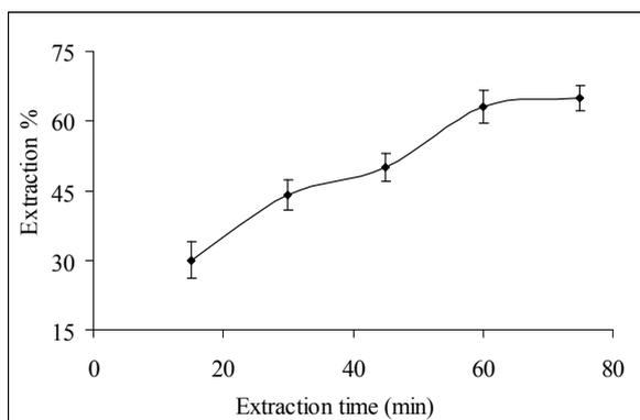
**Figure 3.** The effect of time on the extraction efficiency. Extraction conditions:  $C_{TAM}$ ,  $50 \text{ ng}\cdot\text{mL}^{-1}$ ; SP,  $15 \text{ mL}$  of  $0.01 \text{ M NaOH}$  (pH 11.8); RP,  $25 \mu\text{L}$  of  $0.01 \text{ M}$  phosphate buffer (pH 2.0); stirring rate,  $1000 \text{ rpm}$ .
