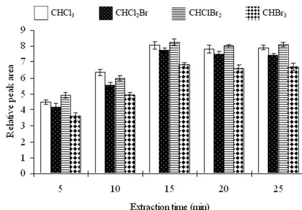
**Figure 4.** Influence of the extraction time on the extraction efficiency. Extraction conditions as with Fig. 3 and: 3 M of NaCl, extraction solvent (1-undecanol) volume of 7.0  $\mu\text{L}$  with stirring rate of 750 rpm.
