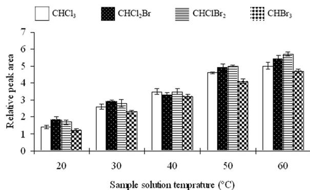
**Figure 2.** Influence of the aqueous sample temperature on the relative peak area. Extraction conditions as with Fig. 1 and extraction solvent: 1-undecanol.
