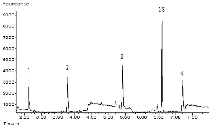
**Figure 5.** Chromatogram obtained by GC-MS after performing LPME of tap water one, spiked with THMs (0.50  $\mu\text{g/L}$ ). Peak numbers correspond to (1)  $\text{CHCl}_3$ , (2)  $\text{CHCl}_2\text{Br}$ , (3)  $\text{CHClBr}_2$ , I.S.: Internal standard-1, 2-dibromopropane, and (4)  $\text{CHBr}_3$ .
