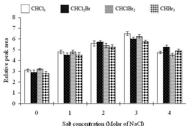
**Figure 3.** Effect of the salt addition on the relative peak area. Extraction conditions as with Fig. 2 and aqueous sample temperature 60°C.
