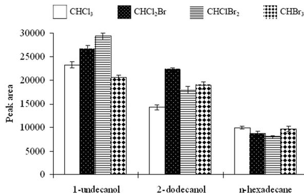
**Figure 1.** Effect of the organic solvent type on the extraction efficiency. Conditions: sample volume: 10.0 mL; extraction temperature: 60°C; extraction solvent volume: 10.0 µL; stirring rate: 600 rpm; extraction time: 25 min, and without salt addition.
