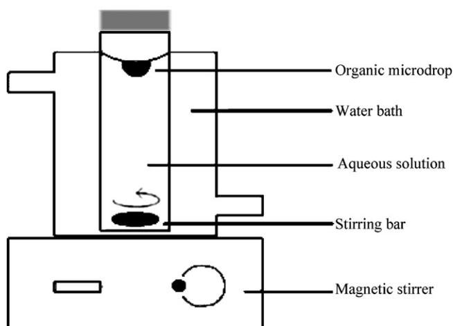
**Fig. 1 – Schematic diagram of the proposed LPME apparatus.**
