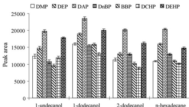
**Fig. 1.** The effect of the organic solvent type on the extraction efficiency. Conditions: sample volume, 10.0 mL; extraction temperature,  $60^\circ\text{C}$ ; extraction solvent volume,  $10.0 \mu\text{L}$ ; stirring rate, 600 rpm; extraction time, 30 min, and without salt addition.
