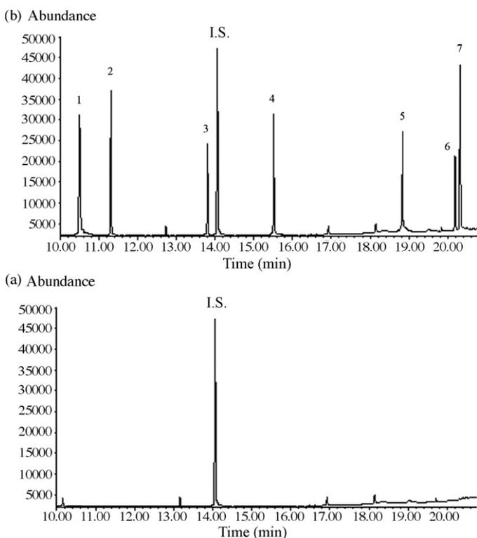
**Fig. 5.** The chromatograms obtained by GC-MS of the mineral water (Cheshmeh) after performing LPME, without spiking PEs (a) and spiked with PEs (b) at the concentration level of 5.0  $\mu\text{g L}^{-1}$  of each analyte. Peak numbers correspond to (1) DMP; (2) DEP; I.S.: benzyl benzoate; (3) DAP; (4) DnBP; (5) BBP; (6) DCHP; (7) DEHP.
