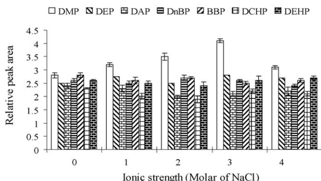
**Fig. 2.** The effect of the salt addition on the relative peak area. Extraction conditions as with Fig. 1, extraction solvent: 1-dodecanol.
