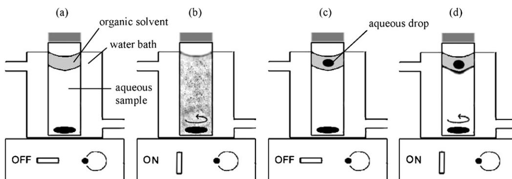
Fig. 1. Directly suspended droplet LLLME setup.
