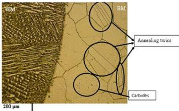
Fig.4. Annealing Twins and Carbides in Base Metal
